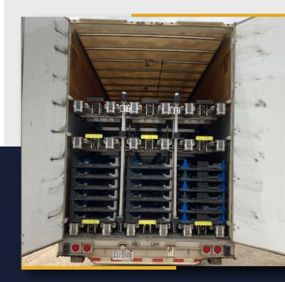
The image above shows the inside of one of BWI's custom spec-ed trailers. These trailers are designed specifically to deliver the right automotive part at the right time during manufacturing sequences.
